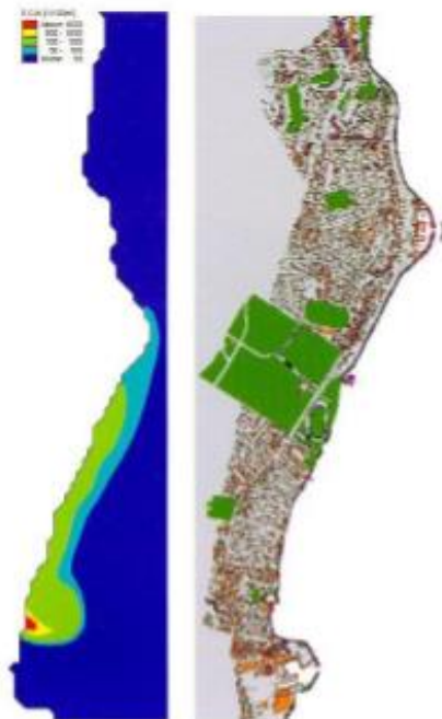
Example of bathing water quality forecasts from a municipality north of Copenhagen. The forecasts are made available on a dedicated bathing water quality webpage
