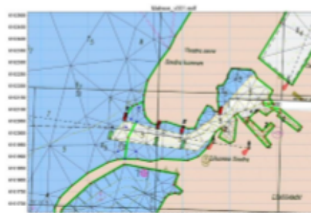
Example of Flexible Mesh generated for a flushing study in Port of Malmoe, Sweden. The background image is from MIKE C-Map which enables extraction of land contours and water depths from digitized Admiralty Charts provided by Jeppesen Norway
